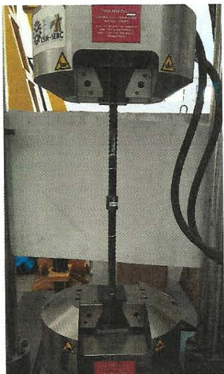
Fig. 9 Close-up view of low cycle fatigue test on a reinforcing bar coupler of 25 mm diameter
