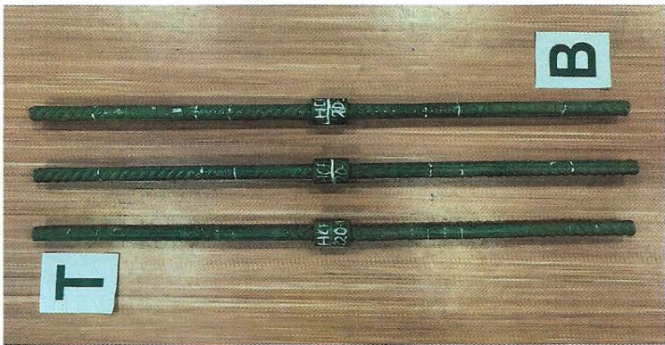
Fig. 4 Reinforcing bar couplers of 20 mm diameter after completion of high cycle fatigue tests
