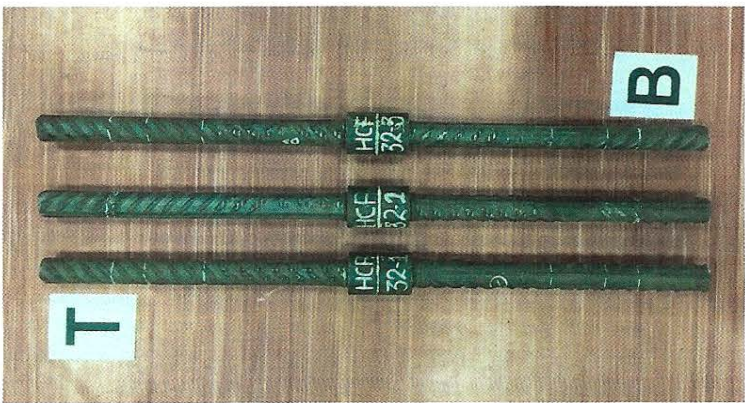
Fig. 12 Reinforcing bar couplers of 32 mm diameter after completion of high cycle fatigue tests
