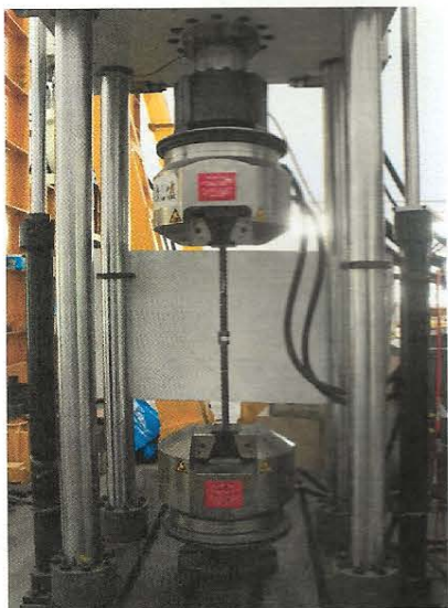
Fig. 6 Test set-up for low cycle fatigue test on a reinforcing bar coupler of 20 mm diameter
