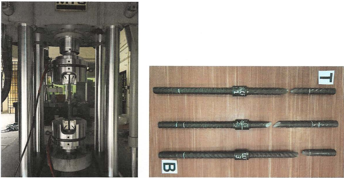
Fig. 5 Failure pattern of 32 mm diameter reinforcing bar couplers observed during static tensile tests after low cycle fatigue tests
