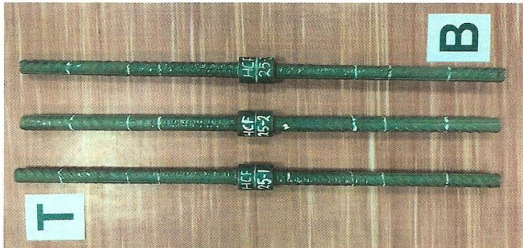
Fig. 8 Reinforcing bar couplers of 25 mm diameter after completion of high cycle fatigue tests
