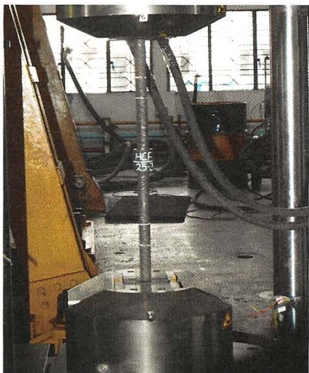
Fig. 6 Close-up view of high cycle fatigue test on a reinforcing bar coupler of 25 mm diameter
