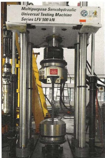
Fig. 1 Set-up for low cycle fatigue test on a reinforcing bar coupler of 32 mm diameter
