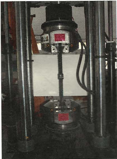
Fig. 1 Test set-up for cyclic tensile test on a reinforcing bar coupler of 32 mm diameter
