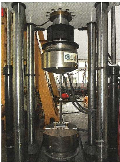
Fig. 2 Close-up view of high cycle fatigue test on a reinforcing bar coupler of 20 mm diameter
