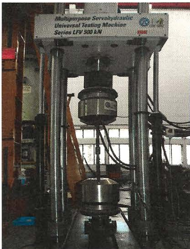
Fig. 9 Set-up for high cycle fatigue test on a reinforcing bar coupler of 32 mm diameter
