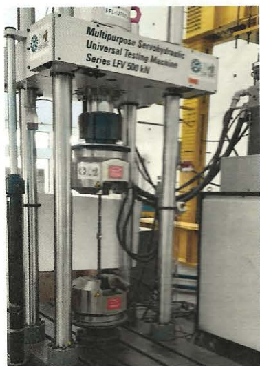
Fig. 8 Test set-up for low cycle fatigue test on a reinforcing bar coupler of 25 mm diameter
