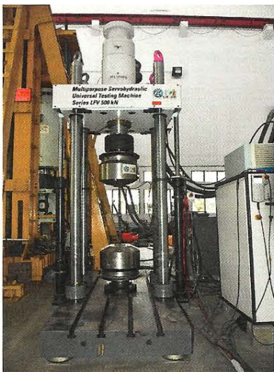
Fig. 1 Set-up for high cycle fatigue test on a reinforcing bar coupler of 20 mm diameter
